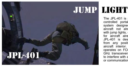
The JPL-401 is a wireless, RFcontrolled portable jump light system designed for use on aircraft not already equipped with jump lights, or as a back-up for aircraft already equipped. JPL-401 is designed to work from any position within the aircraft interior. The system operates on FCC-approved 2.4 GHz transceivers designed not to interfere with aircraft electrical or communication systems.
